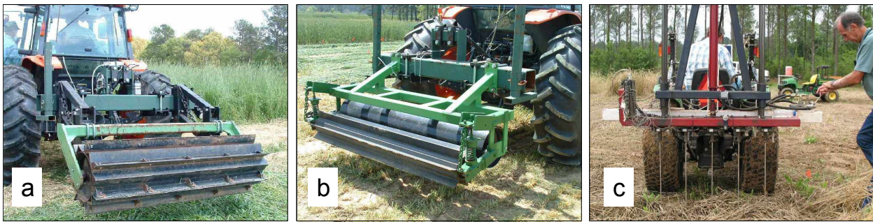
Figure 1. (a) Straight-bar roller; (b) Two-stage roller/crimper; (c) Tractor-mounted penetrometer.
